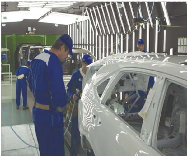
EXAMPLE IMAGES OF TOPCOAT ULTRA-FINE SANDING AND POLISHING TO REMOVE PROCESS INTRUSION DIRT NIBS - FACTORY AND BODY SHOP
