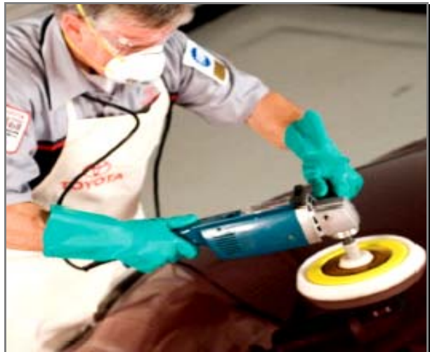
EXAMPLE IMAGES OF TOPCOAT ULTRA-FINE SANDING AND POLISHING TO REMOVE PROCESS INTRUSION DIRT NIBS - FACTORY AND BODY SHOP
